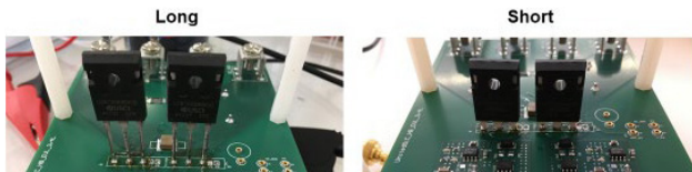
Figure 4. Long Lead (Left) vs. Short Lead (Right). Short Lead is Recommended Whenever Possible.
