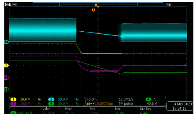
Figure 47. Voltage Transition from 28 V to 9 V at 0.2 A (ch1-Vcc-pwm, ch2-Vds-sec, ch3-Vc58, ch4-Vo)
