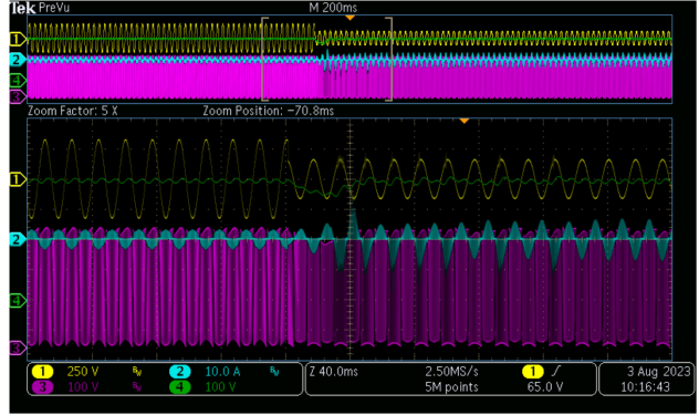
Figure 22. 230 Vac to 115 Vac Transition at Full Load (ch1-Vin, ch2-IL, ch3-Vfast leg SW, ch4-Vbulk)
