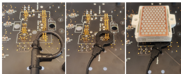
Figure 11. Mounting Detail Rogowski Coil to PCB
