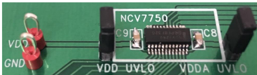
Figure 12. UVLO Jumper and VDD Test Post Locations
