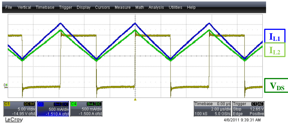
Figure 4. Operational Waveforms, V_{IN} = 12\text{ V} , R_{OUT} = 6\ \Omega
