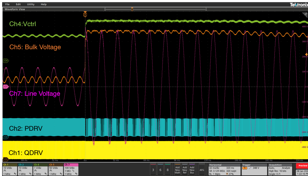
Figure 15. 90 Vac to 264 Vac Line Transition
