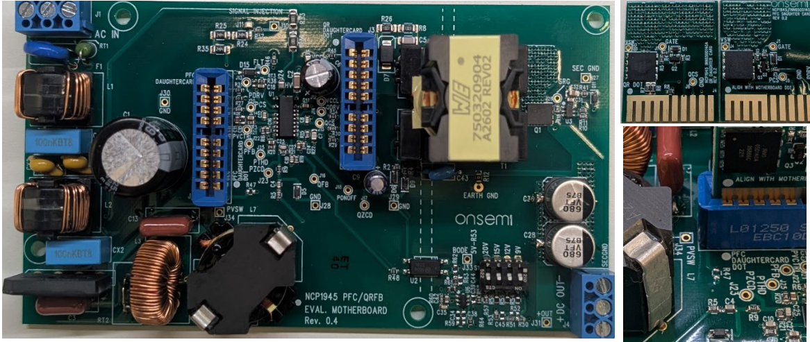
Figure 6. NCP1945 USB-PD Evaluation Board and Daughter Cards
