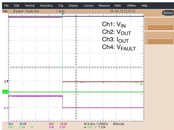
Figure 22. Short Circuit Event on Latching Device
