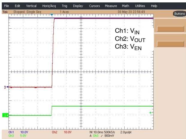
Figure 16. Turn On with EN Pin with C_{dvd1} Open
