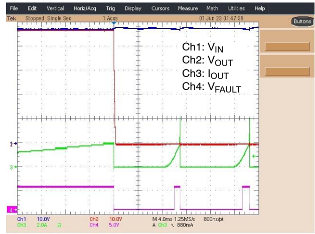
Figure 19. I_{TH} Overcurrent Event on Auto-retry Device
