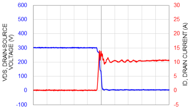
Figure 10. Turn-on Waveform Tj = 100 °C, VPN = 300 V
