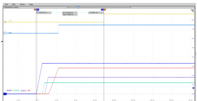
Figure 15. Power-up Sequence Example of the AA Version, See Power Sequence on Page 19 for more Details
