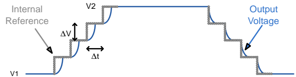
Figure 44. DVS in Forced PPWM Mode Diagram
