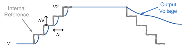
Figure 45. DVS in Auto Mode Diagram
