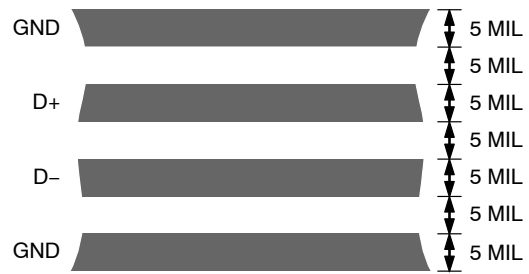
Figure 22. Typical Arrangement of Signal Tracks
