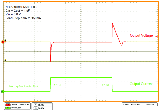
Figure 18. Load Transient Response
