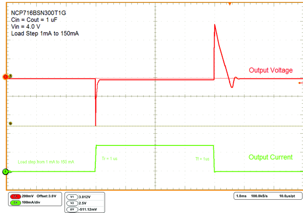
Figure 17. Load Transient Response
