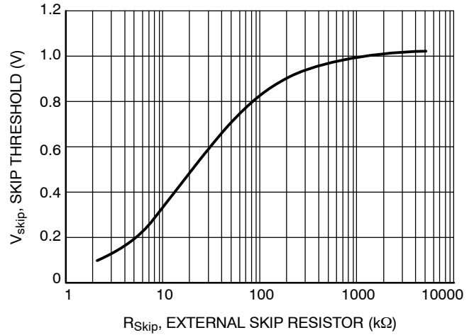
Figure 22. Skip Threshold vs. Skip Resistor
