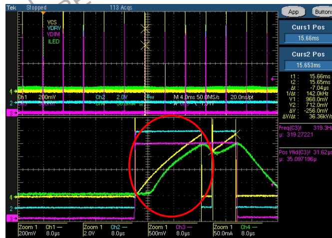
Figure 31. Minimum Dimming Duty Cycle
