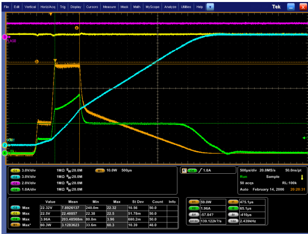
Figure 3. V_{IN} = 22\text{ V} , C_{SS} = 5.6\text{ nF} , C_{IN} = 10\text{ }\mu\text{F} , C_{OUT} = 250\text{ }\mu\text{F}
